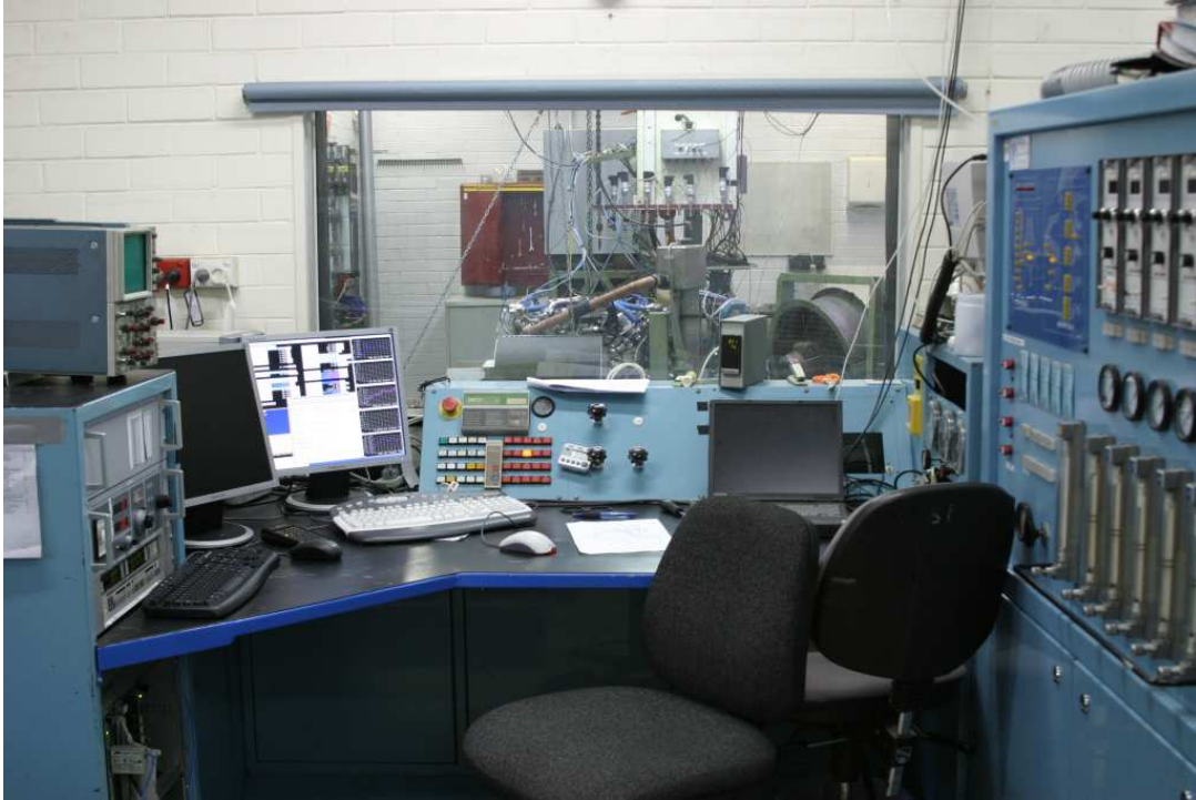
Figure 3.2. Engine test cell control bench
